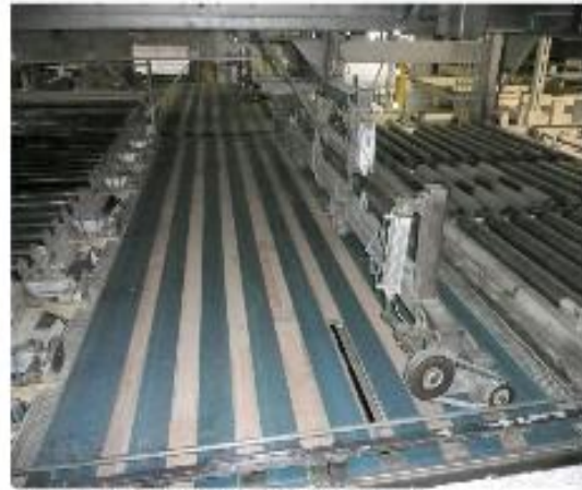
Assembling table with paper feeding vacuum ledge
